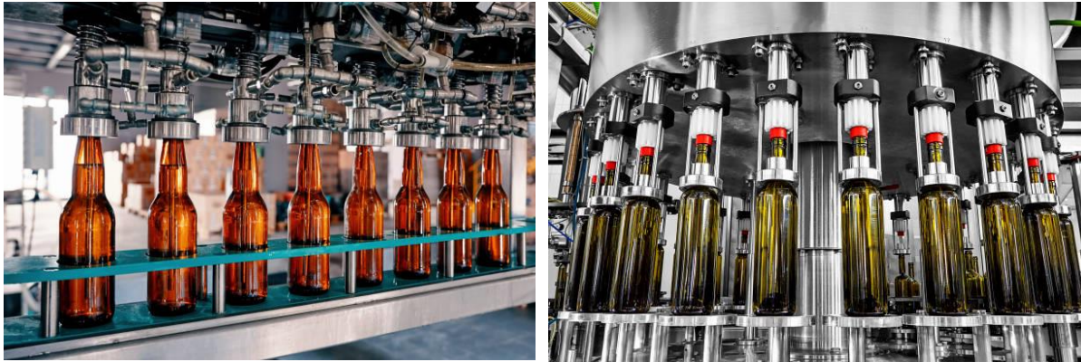
Figure 2: Dossing and capping processes
